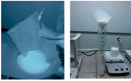
Fig. 1 \text{CaSO}_4 sample preparation using precipitation method.
