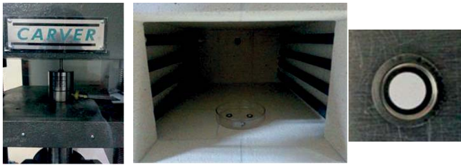
Fig. 2 Pelletizing and sintering of \text{CaSO}_4 samples.
